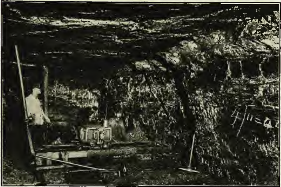
FIG. 145. — Miners working far underground in a bituminous coal mine near Pittsburg. The machine, in front, is drilling a hole in the thick coal seam that forms the wall on the right.
